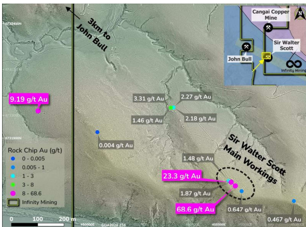
Figure 10: Sir Walter Scott rock chip assay results showing new and historical gold assays along the NW-trending structural corridor.
