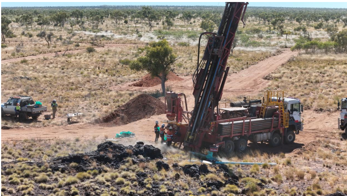
Figure 2. Precision Exploration Drilling’s Reverse Circulation drill rig drilling 26XCRC006 into the discovery outcrop at Kuro.
