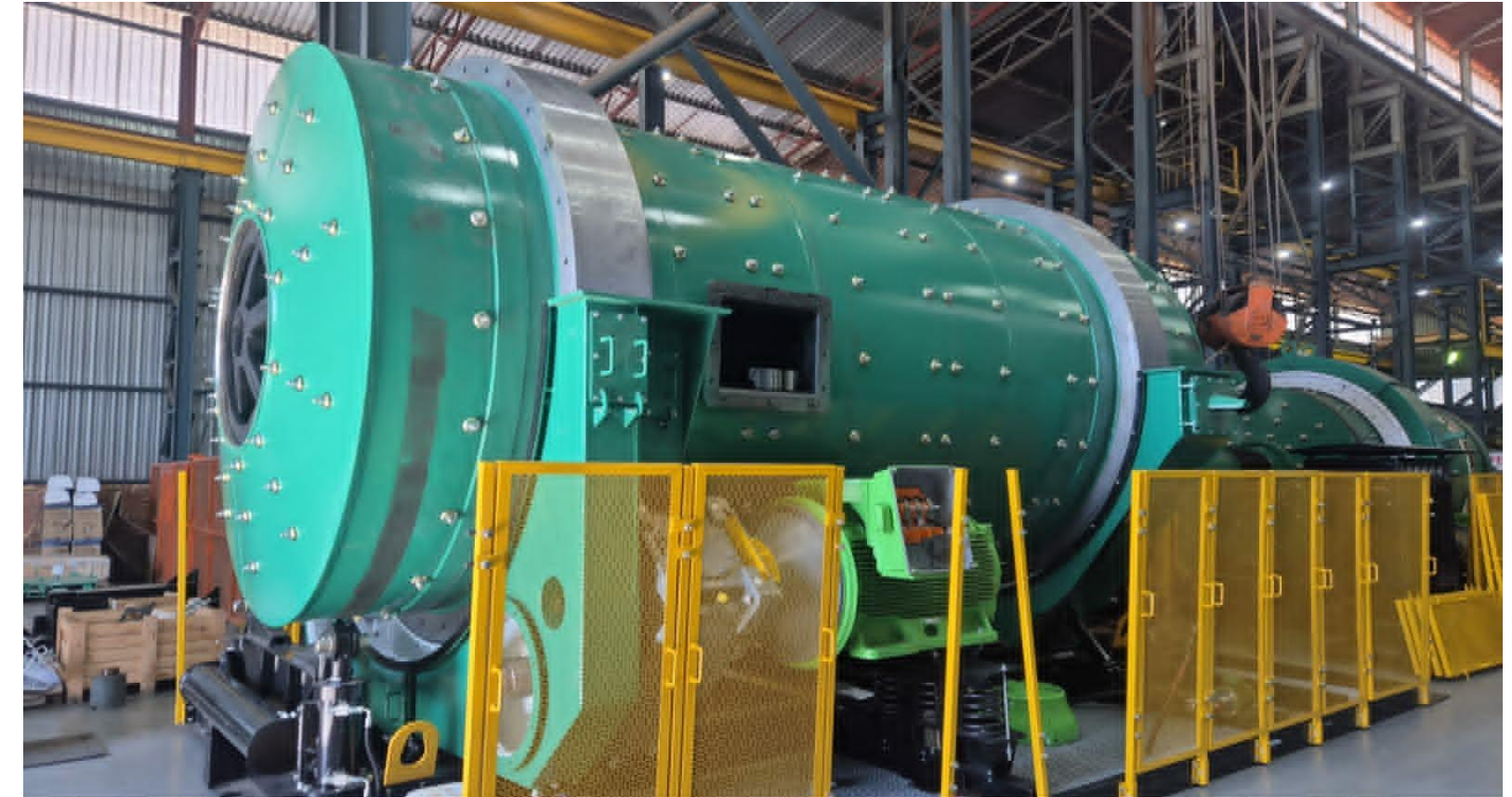
2 x Titan Ball Mill GDM3065 – 900KW
