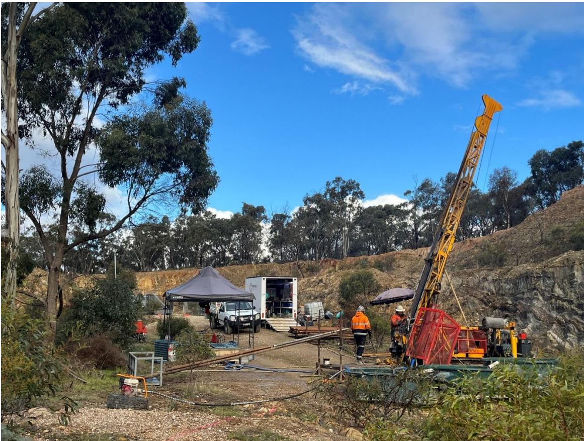
Figure 3 - Diamond Drilling within the Walkers pit at the Comstock Gold Project. Picture taken June 2026 and shows rig targeting shallow depth drilling on the Walkers stockwork vein area and utilizing the existing pit access ramp highlighted in the Concept Study.
