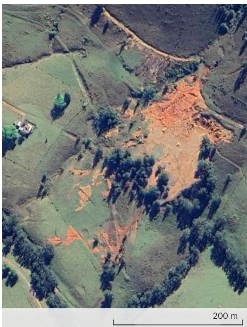
Figure 1: Aerial Image of Remnant Smelter Waste at Cangai
