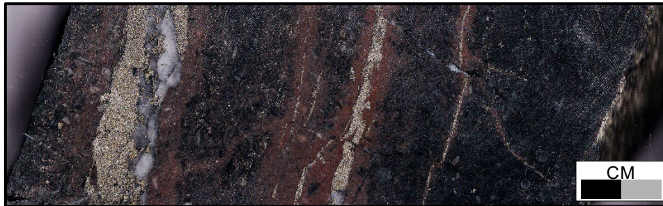
Figure 7: SPD057 – 305.6m, 2.42 g/t Au . Basalt with quartz-chlorite-pyrite veins reactivated by pyrite-chalcopryrite-carbonate veins with potassic selvages
