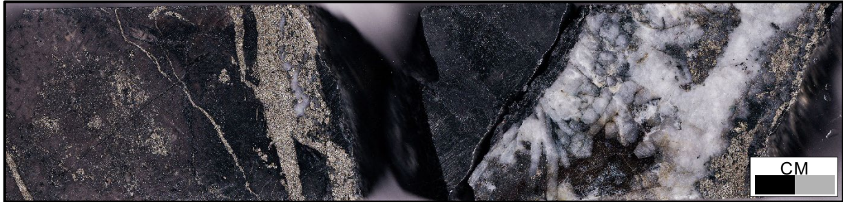
Figure 6: SPD057 – 313.3m, 22.17 g/t Au . Basalt with quartz-chlorite-pyrite veins reactivated by pyrite-chalcopryrite-gold veins and pyrite veinlets
