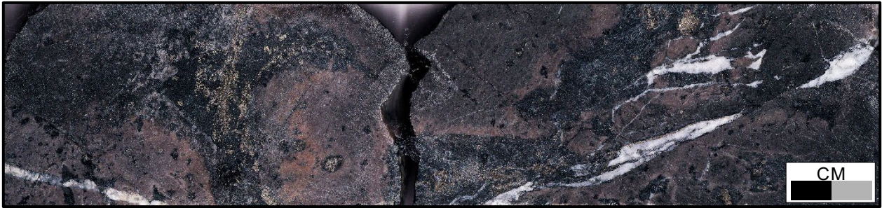
Figure 8: SPD059 – 281m, 4.88 g/t Au . Albitised basalt-andesite with chlorite-chalcopyrite-pyrite crackle breccia infill with potassic selvages and late carbonate veining
