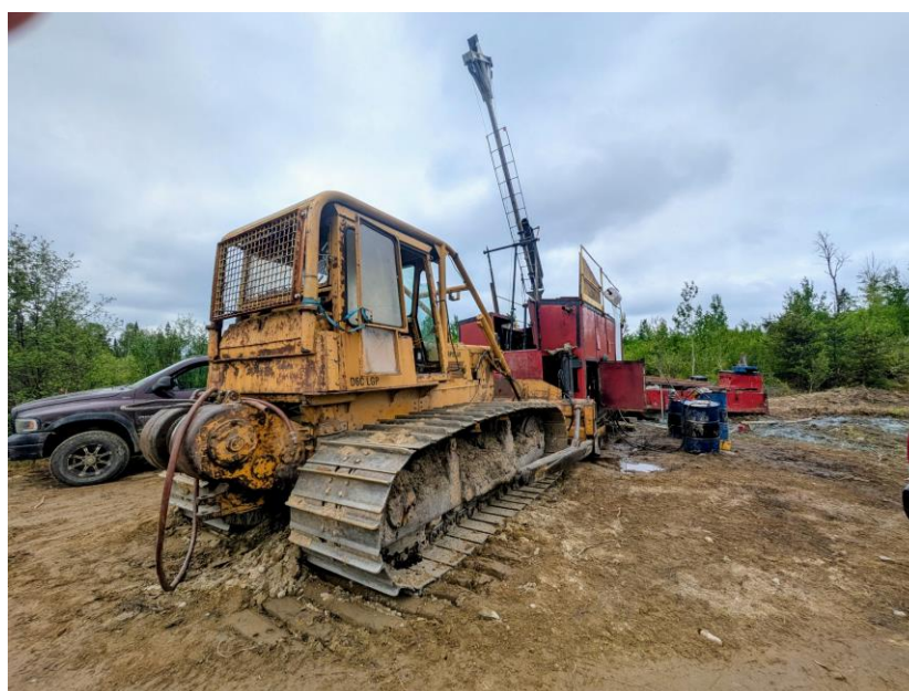
Figure 4: Diamond drill rig at the Shanty Lake target, where the bit is approximately 150m from target.
