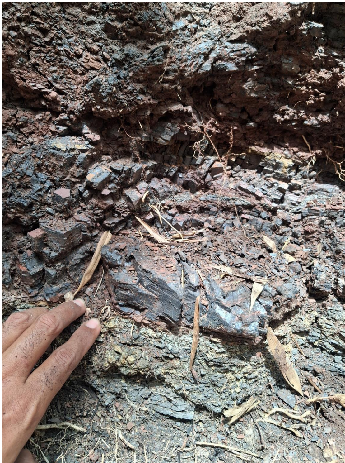
Figure 3: Exposed in-situ Manganese at the Leuro prospect, sampled as ESR006054, assayed 52.8% Mn
