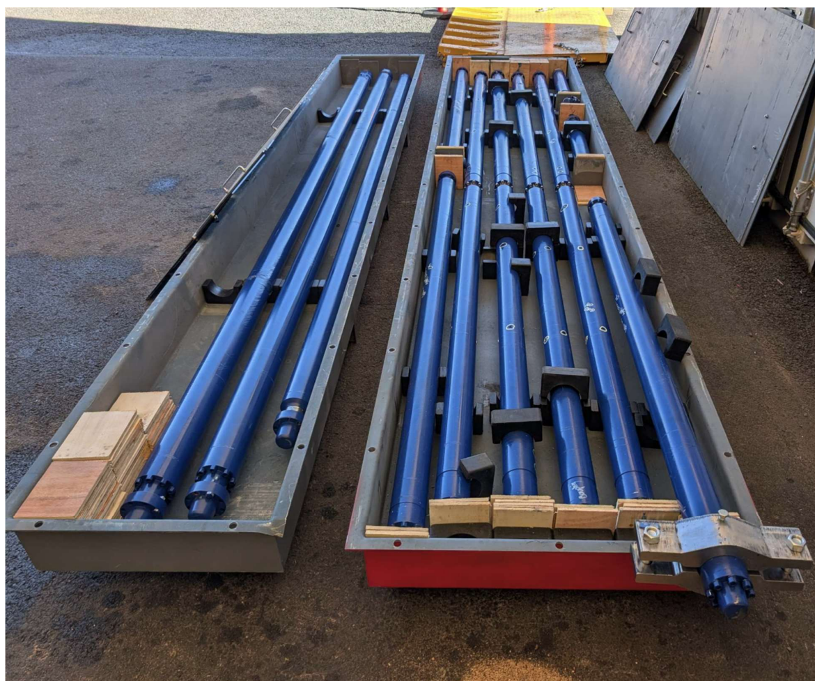
Figure 3: Electric Submersible Pump (ESP) for Ramsay 1 and Ramsay 2 well flow test rated to a maximum fluid flow rate of 2,000bbl/day undergoing factory acceptance tests
