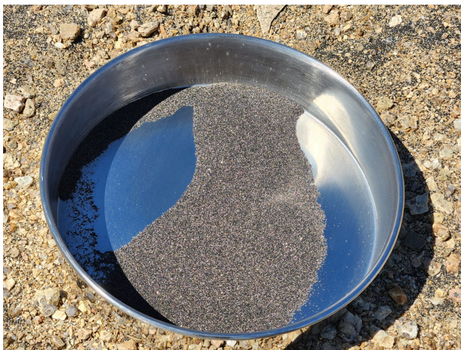
Figure 7. Sieved heavy mineral concentrate (<200 \mu\text{m} ) collected from eastern drainage systems for laboratory analysis.
