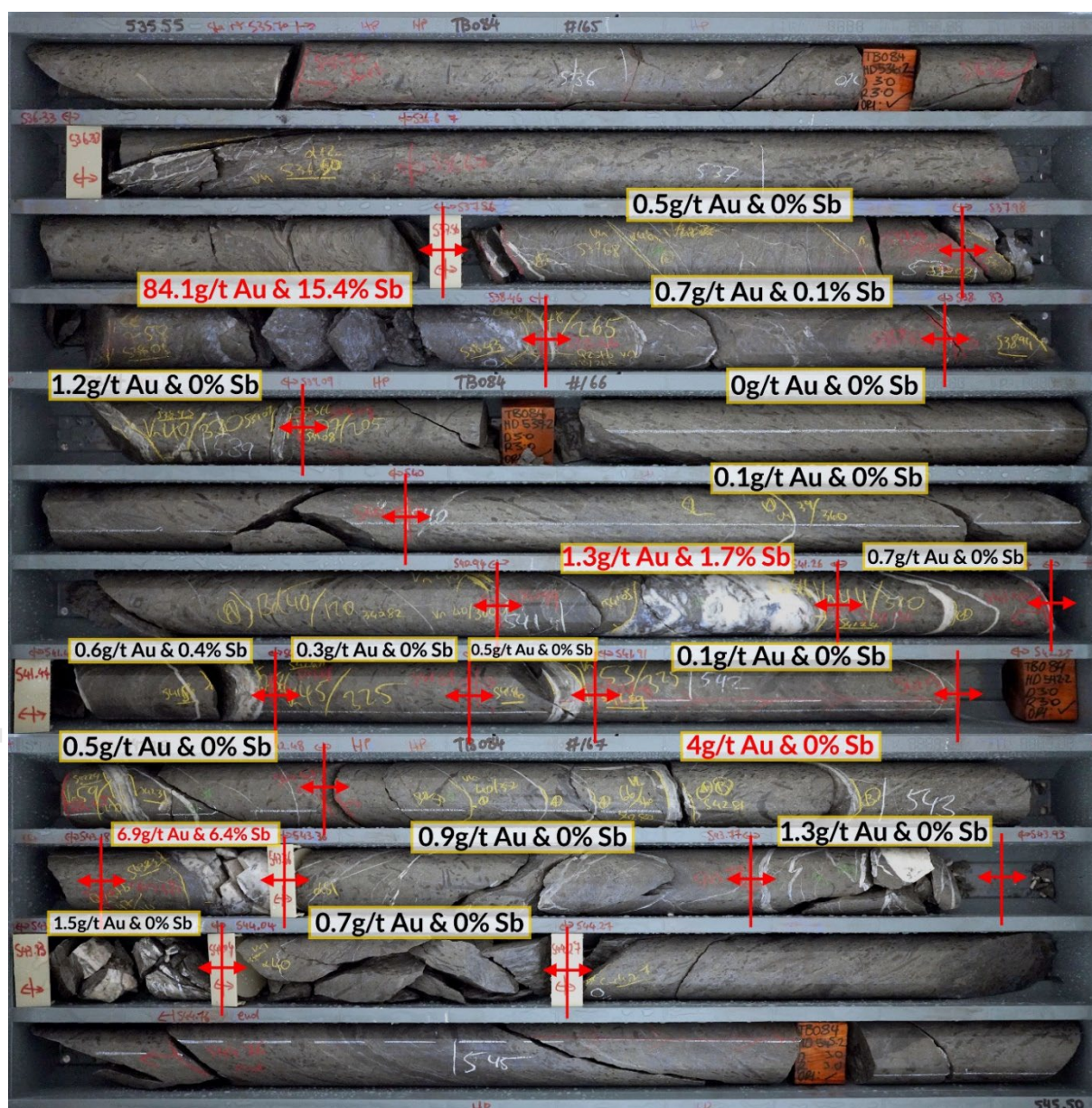
Figure 7. Core tray photograph of the Freeman-702 vein splay zone intersected in TB084, where the highest grade interval of the drill program was intersected.
