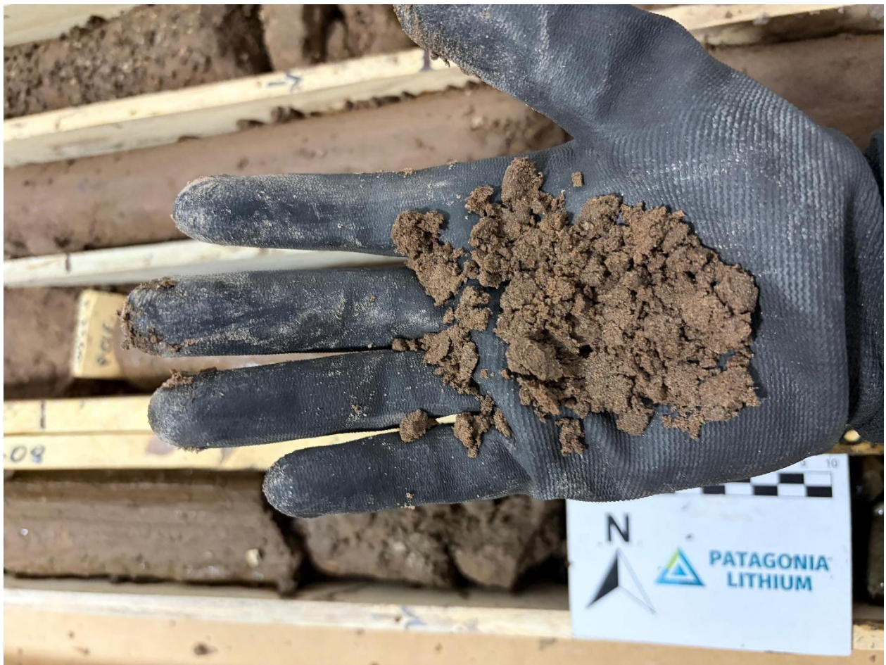
Figure 1. JAM 26-08 Cilon core sample gravels (top left hand corner) and sand contributing to high porosity.
