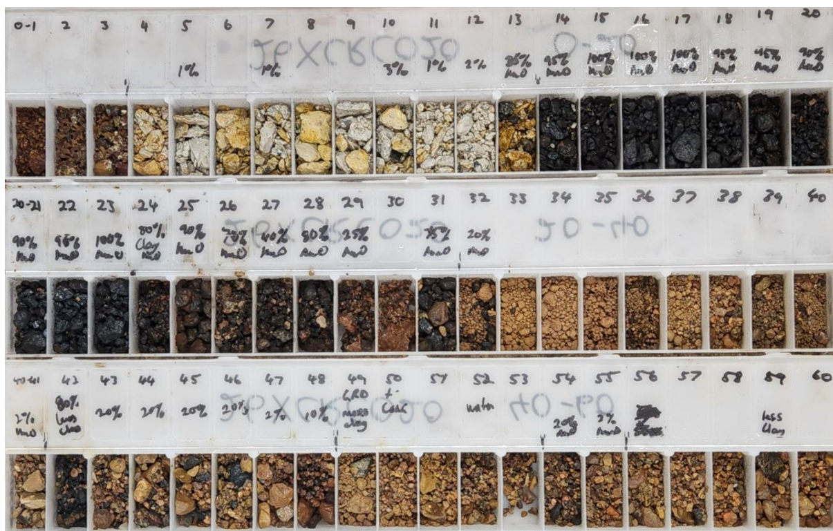
Figure 4. 26XCRC020 chip tray photo, showing interpreted visual manganese mineralised interval, with 10 metres of visual massive manganese from 13m down-hole, within a broader zone of 17 metres from 12m down-hole, and 2 meters of visual semi-massive manganese from 30m down-hole. Readers are referred to Table 2 for detailed information regarding visual estimates. Corresponding sample IDs are: TKMRC02521 – 2585.
