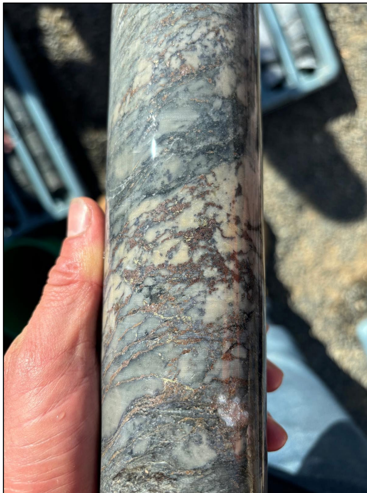
Figure 5: A3DD013 at 440m stringer sulfide veins of sphalerite (brown) chalcopyrite (yellow) from mineralised zone grading 2m at 2.7% Zn+Pb, 0.1% Cu from 439m
