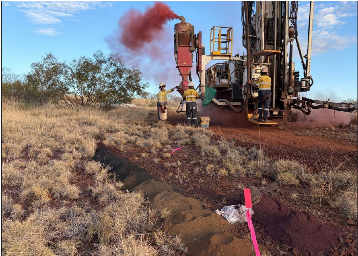
Figure 2. RC drill hole being completed (WDRC311') that intersected 6m @ 31.5% Mn from 3m and 3m @ 57.5% Fe from 10m.
