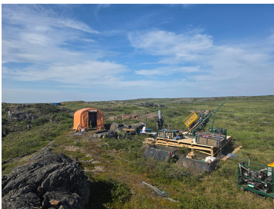
Figure 3: Photograph of reverse circulation drilling rig at JWS26001. Drillhole is targeting the historic "discovery zone" and will confirm the core of the known mineralisation
