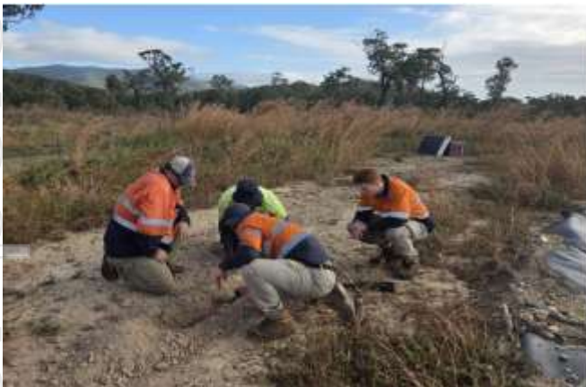
Figure 1 – Zonge field crew digging in sensors for the Dittmer MT survey.
