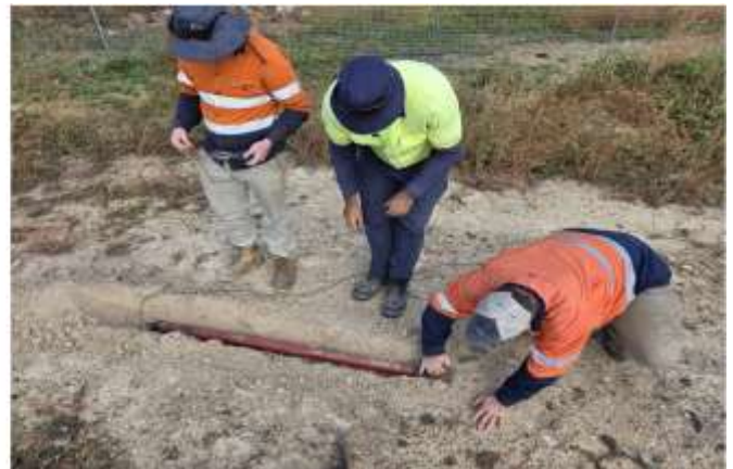
Figure 1 – Zonge field crew digging in sensors for the Dittmer MT survey.
