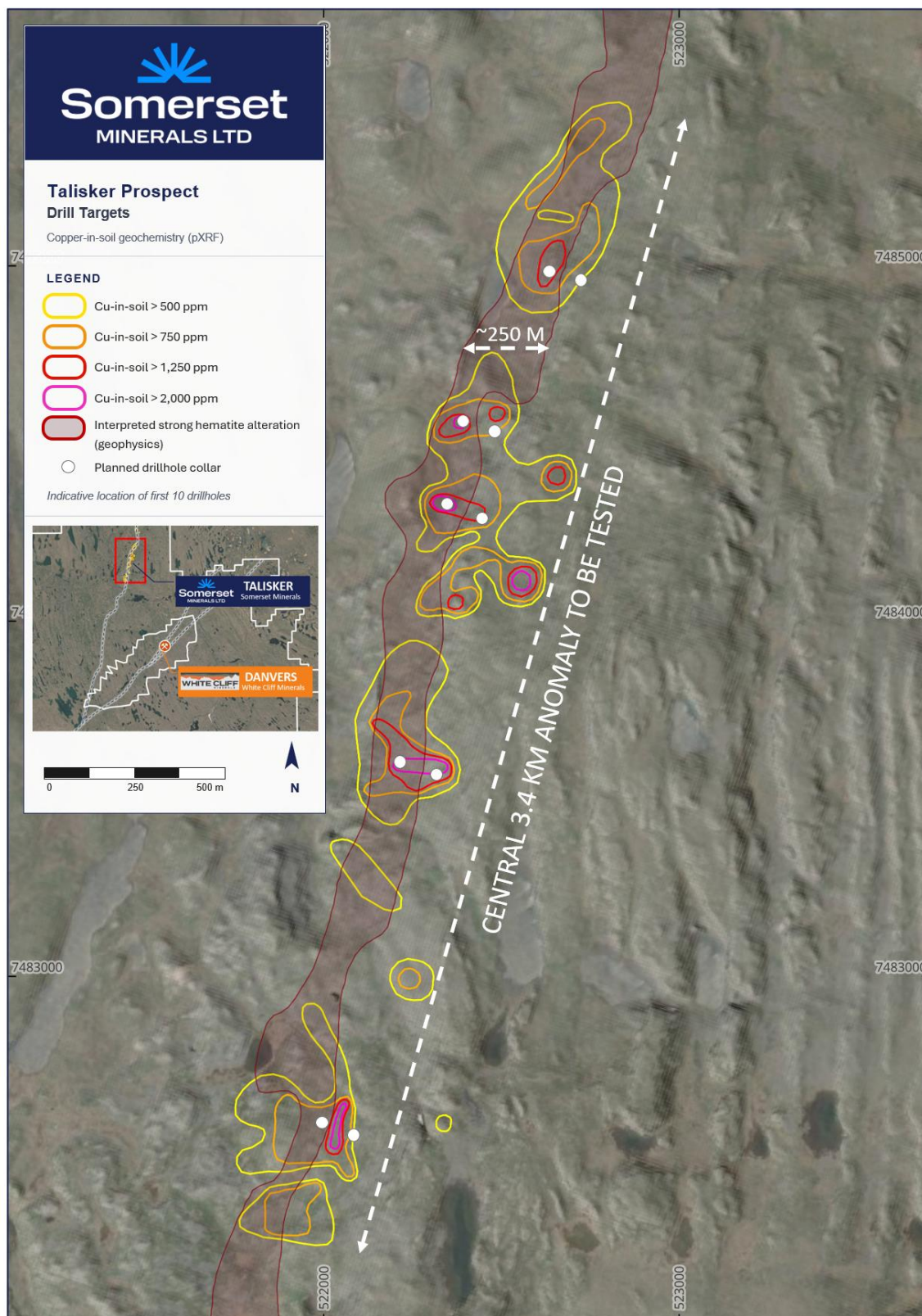
Figure 1: Upcoming drill targets on the 3.4km-long newly refined Talisker anomaly, part of the 17-km long anomaly identified from regional geochemistry in 2025. Highly anomalous copper in soils is associated with a large demagnetised linear feature, interpreted to represent intense hematite alteration produced by hydrothermal mineralising fluids along the Talisker fault.
