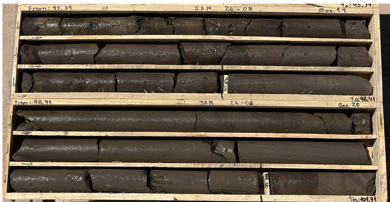
Figure 2. Black sands encountered at 98-101m depth.
