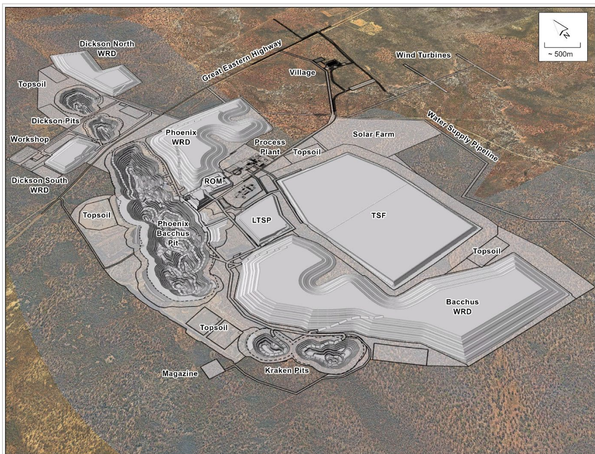
Figure 21: Bullabulling Gold Project infrastructure layout
