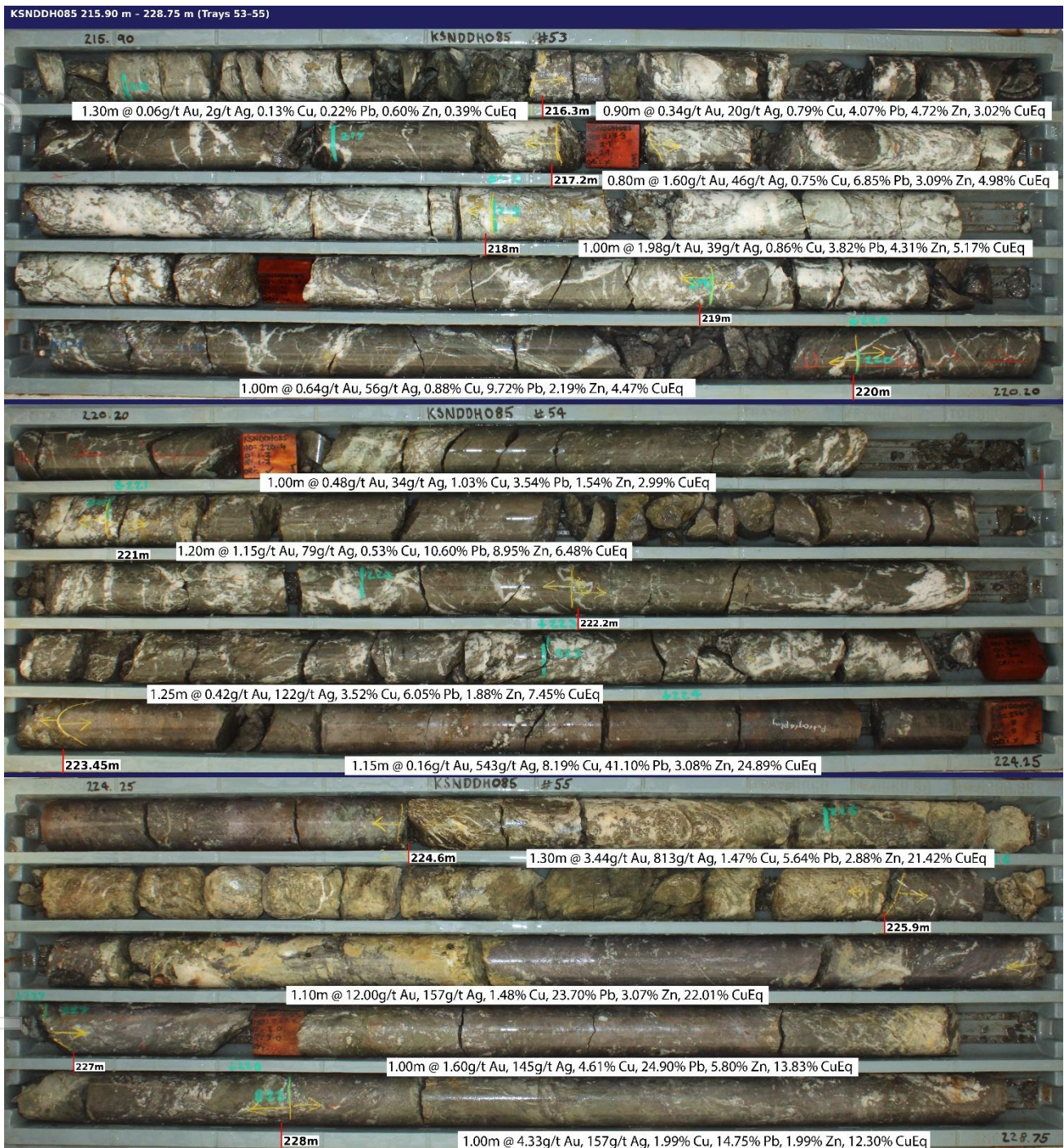
Figure 3: KSNDH086 drill core, 215.90m to 228.85m. Tray 53 contains abundant epithermal veining with high grades for gold, copper, lead, zinc and silver. In Tray 54, high grade base metal and silver mineralisation starts from 223.45m and continues into Tray 55.
