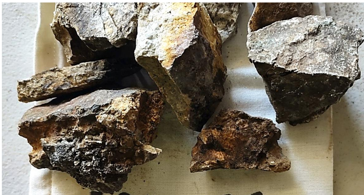
Figure 4: Sample 3017023, best Au sample (12.3ppm) has narrow zones of gossanous breccia (lower) with anomalous Cu Ag Bi Mo S in albite altered porphyry (upper).
