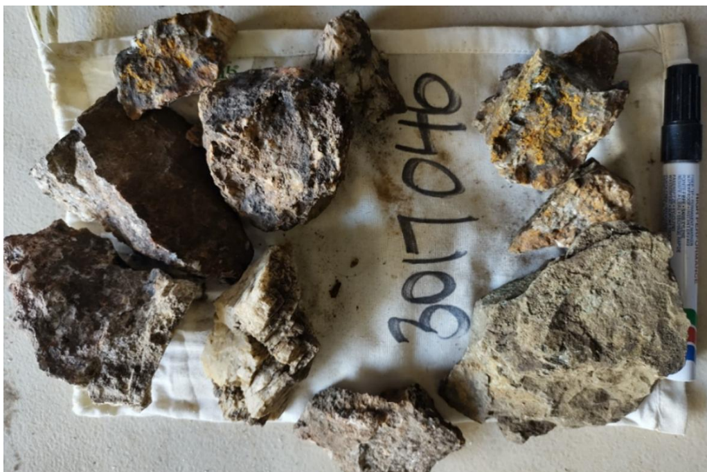
Figure 6: Sample 3017046, the best Cu sample (10900ppm) has dark gossanous breccia zones with jarosite limonite and chalcocite in cavities in fractured and brecciated buck quartz.
