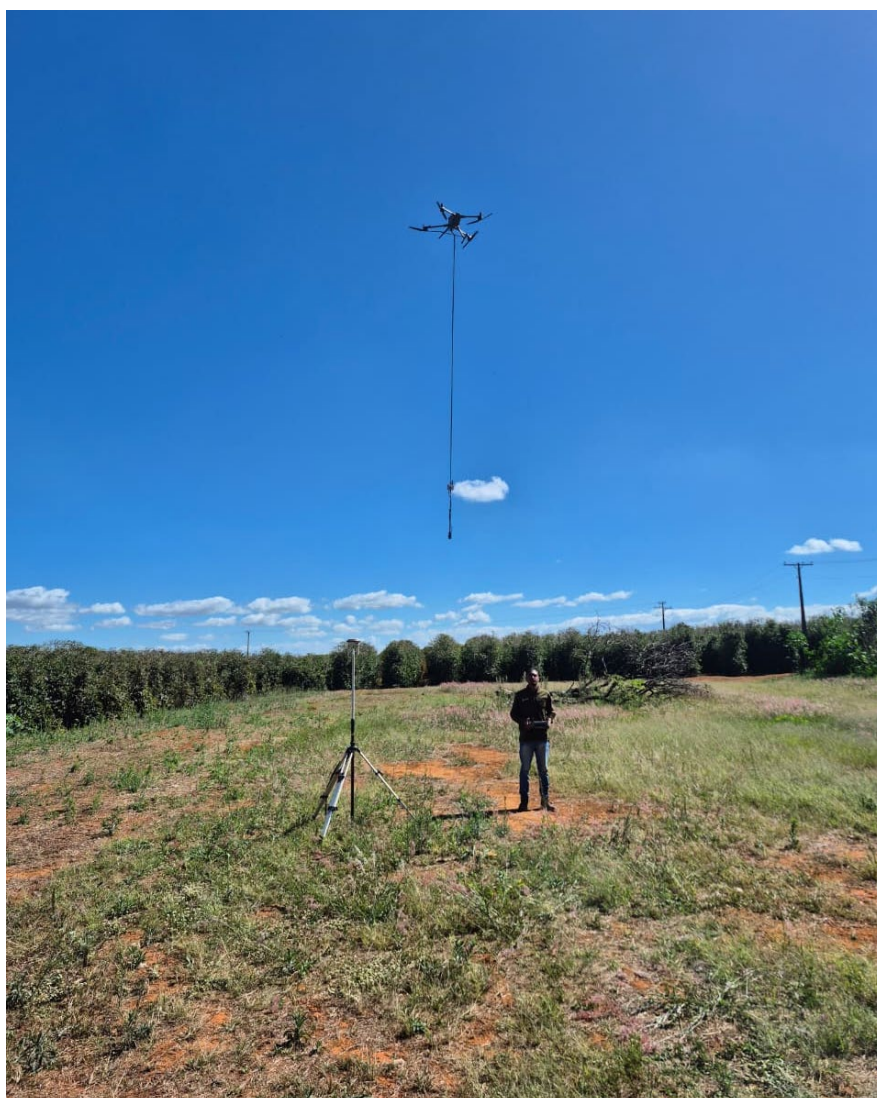
Figure 6. Drone geophysical surveys underway at Serra Negra. Drone-based geophysical surveys commenced on 29 June 2026. The program comprises high-resolution LiDAR surveying followed by drone magnetic surveying across the priority target areas. Data will be integrated with geological and drilling datasets to refine targeting ahead of the initial drilling campaign.
