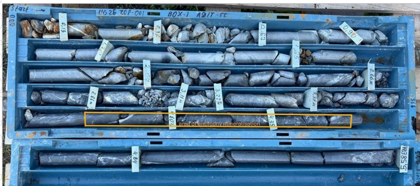
Figure 4 Photo of the mineralised antimony zones (yellow box) within drillhole UG26ZOP-001 showing breccia of quartz with stibnite filling veins and vugs (~10% Stb). Drilling prior to the antimony zone is enriched in arsenopyrite sulphide alteration which may contain gold. Assays are pending for this hole.
