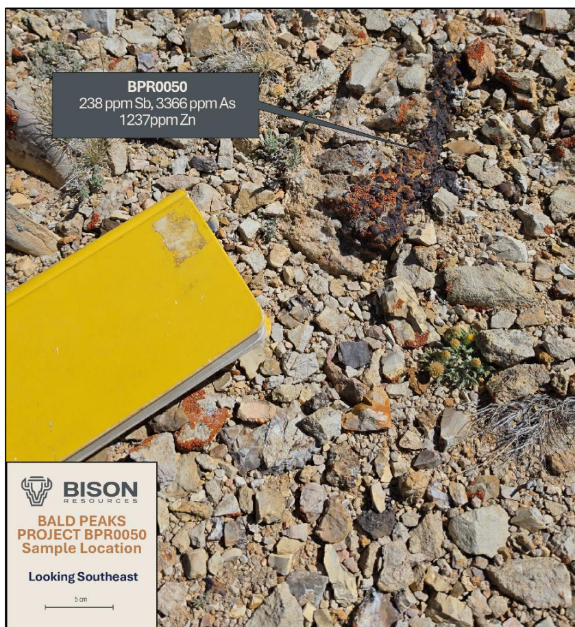
Figure 3: Rock chip sample BPR0050 (660,441mE, 4,460,263mN, 2,373mRL) in-situ subcrop showing iron oxides in carbonate at the Bald Peaks Project.
