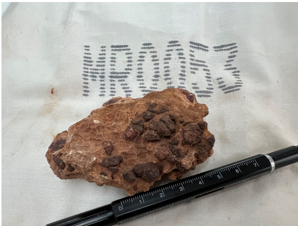
Figure 3. Sample MR0013 (originally MR0053) showing weathered breccia material with dark brown iron-carbonate nodules.
