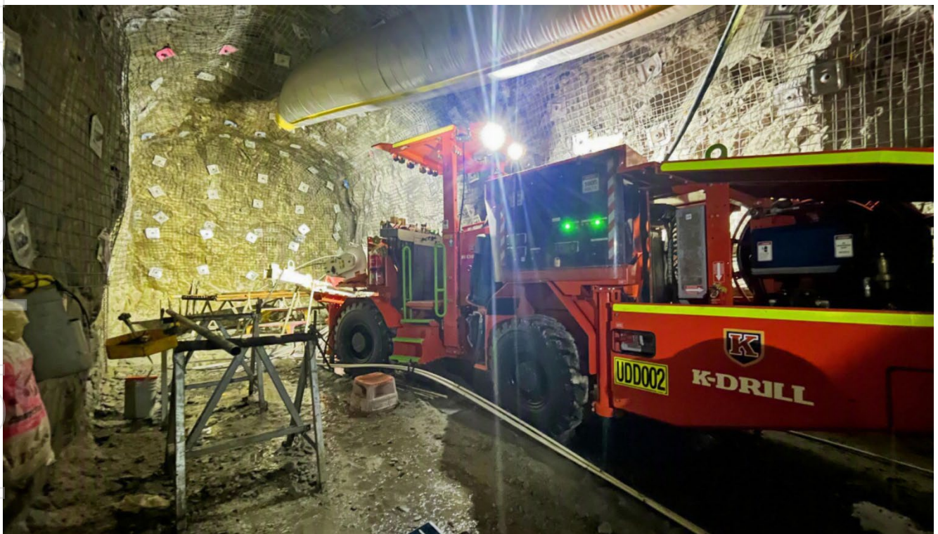
Figure 9 – Diamond Drill rig operating in United North underground
