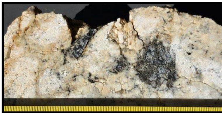
Figure 3 Sample no 105498 (3.04% W). Vein no 3. Field of view approximately 22cm. Coarse patches of biotite and wolframite within a coarse weakly brecciated pegmatitic granite. ASX announcement dated 4 June 2026.
