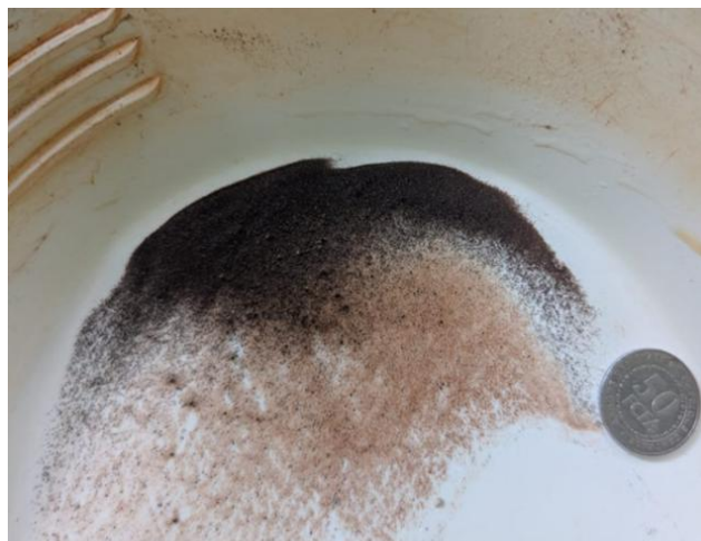
Figure 2: Field photo of a panned sample from Minta 1, showing HM and visible rutile from sample M1S0056. Hole ID M10130 at coordinates 258150 mE / 495000 mN.
