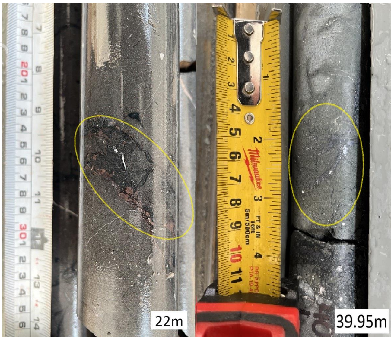
Figure 6 - Photographs of bornite bearing brecciated veins (left) and chalcocite veinlets (right) in variably chlorite and hematite altered basalts from drillhole DAN26026. Yellow ovals depict zones of mineralized cement. Core is NQ2 diameter.
