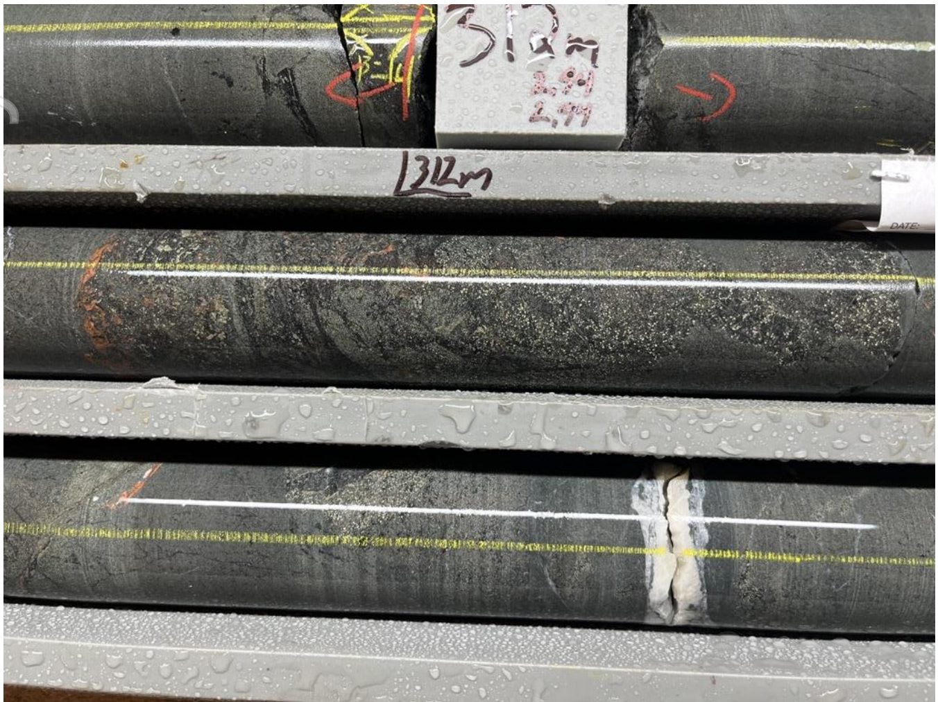
Figure 8 - Zones of disseminated chalcopyrite in DAN26030. Drill core is NQ2 size
