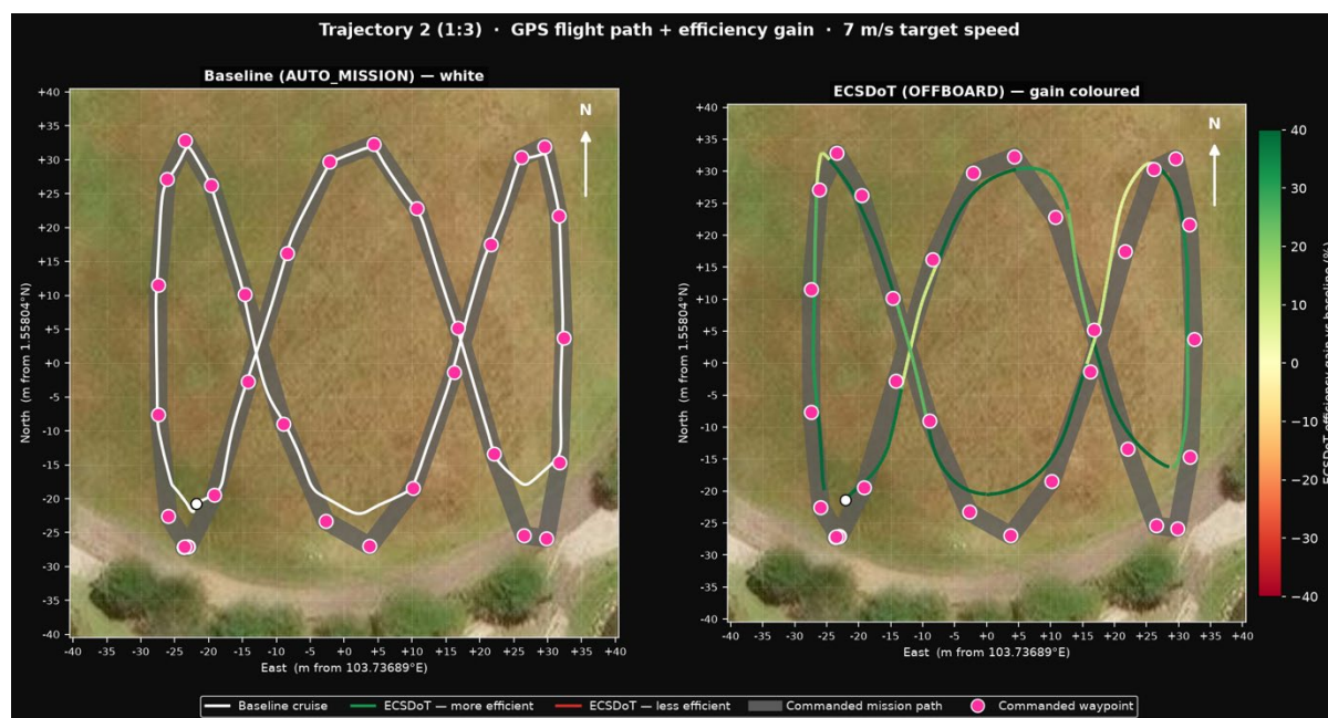
Figure 7: GPS Flight Path Efficiency Overlay: Trajectory 2 (Sinusoidal) at 7 m/s, Baseline (White, Left) vs ECS-DoT Efficiency Gain (Colour-Coded, Right)
