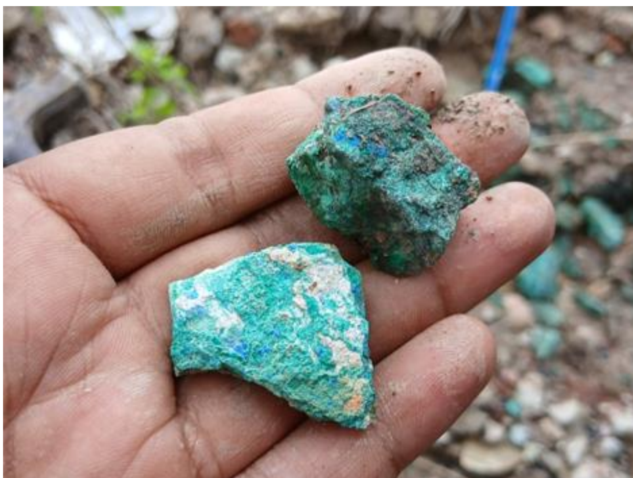
Figure 9: Examples of material sampled as ESR006286, which assayed 12.4% Cu and 77ppm Ag
