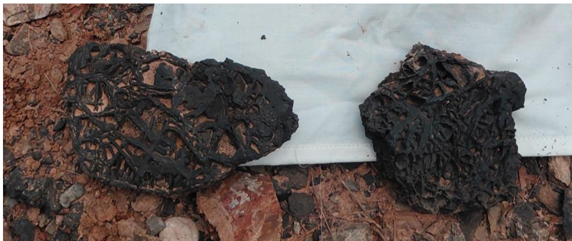
Figure 4: Interpreted gossan displaying boxwork texture, sampled as ESR006094, assaying 26.2ppm Ag Approximately 150m southwest of the copper mineralisation described above, a specimen of oxidised massive sulphide was found (Figures 5 and 6) and sampled as ESR006095.
