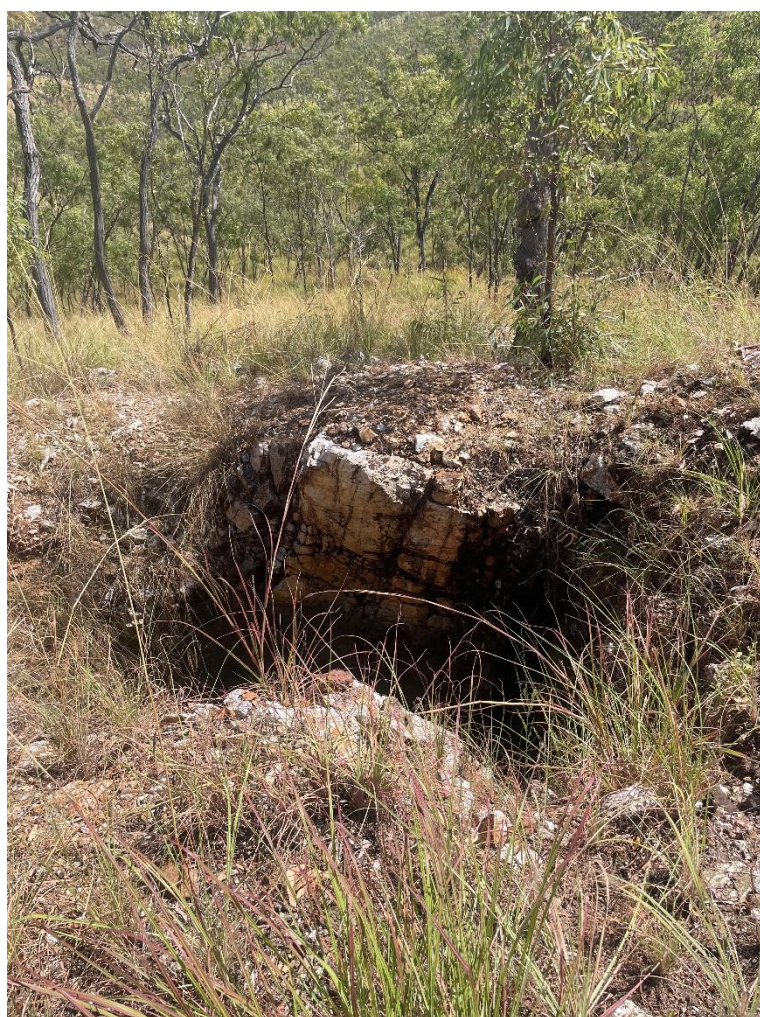
Figure 3 Historic mine spoil at the Lady Burdett Coutts working (~1m wide quartz vein) from which sample P50107 returned 27.3 g/t Au and 12.6 g/t Ag. Associated elevated lead (5,170 ppm), zinc (332 ppm) and cadmium values indicate polymetallic sulphide mineralisation within the quartz vein system. (283183mE, 8135712mN, GDA2020 / MGA Zone 55). Photograph looking west-northwest. Refer to Appendix for JORC Table 1 for the sample results
