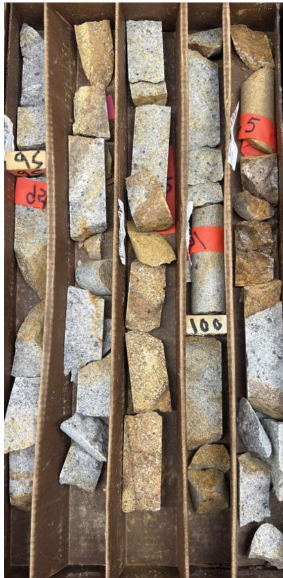
Figure 5: Preserved drill core from hole Cass 06-12 showing quartz-greisen veining with visible cassiterite mineralisation. Laboratory assays over the photographed interval returned 2.29 m @ 0.81% Sn, 1 g/t Ag and 110 ppm W. (Original intercepts 95-98 feet, 3 ft @ 1% Sn, 1g/t Ag, 200 pp W; 98-100 feet, 2 ft @ 0.98% Sn, 1g/t Ag, 50 ppm W; 100-102.5 feet, 2.5 ft @ 0.45% Sn, 2g/t Ag, 50ppm W).
