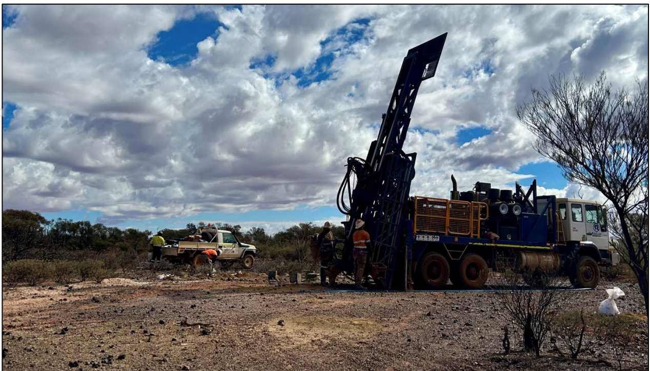
Figure 6: Air core drilling at the Diorama Copper-Gold Target.
