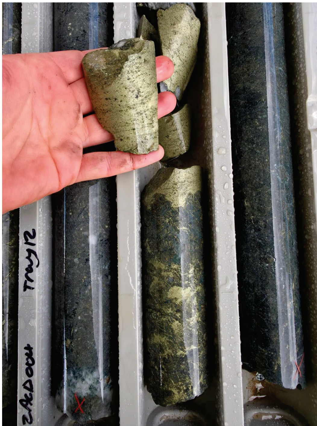
Figure 4: Monza hole MZACD004. Chalcopyrite and pyrite sulphide breccia within potassic altered monzodiorite porphyry. 0.99g/t Au & 4.1% Cu.
