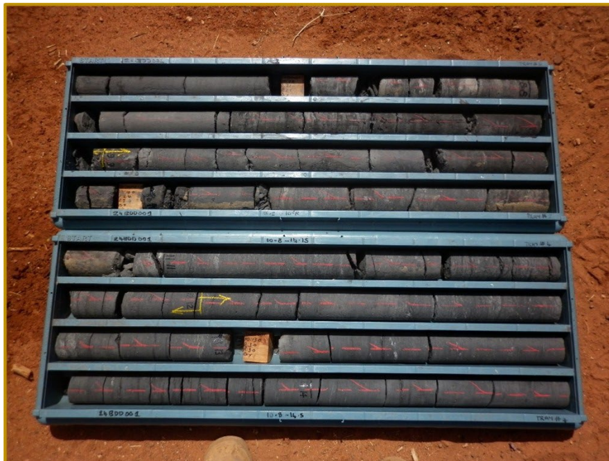
Figure 12. Byro Core Tray (Drillhole 24BDD002 Depth 7.2 – 14.15m) showing Permian Black Shale (refer ASX announcement 25 February 2025)
