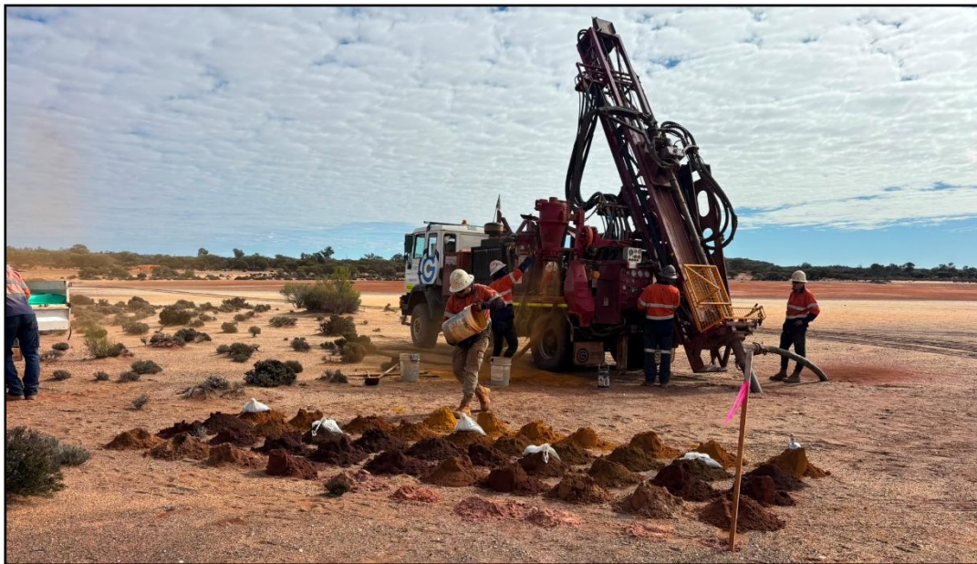
Figure 1. Aircore drilling at the Hastings Gold Prospect.
