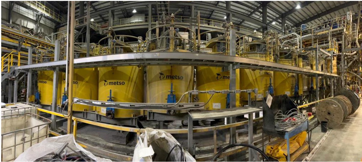
Figure 5. Port MacKenzie flotation cells
