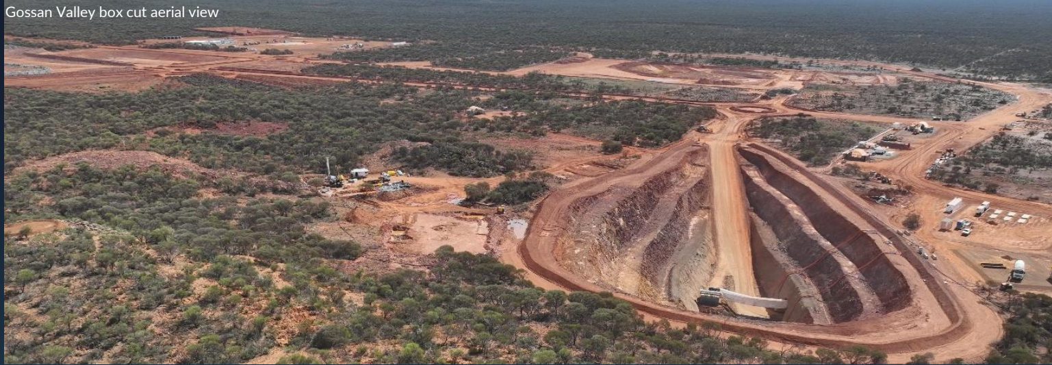
Gossan Valley box cut and decline development - looking north-east
