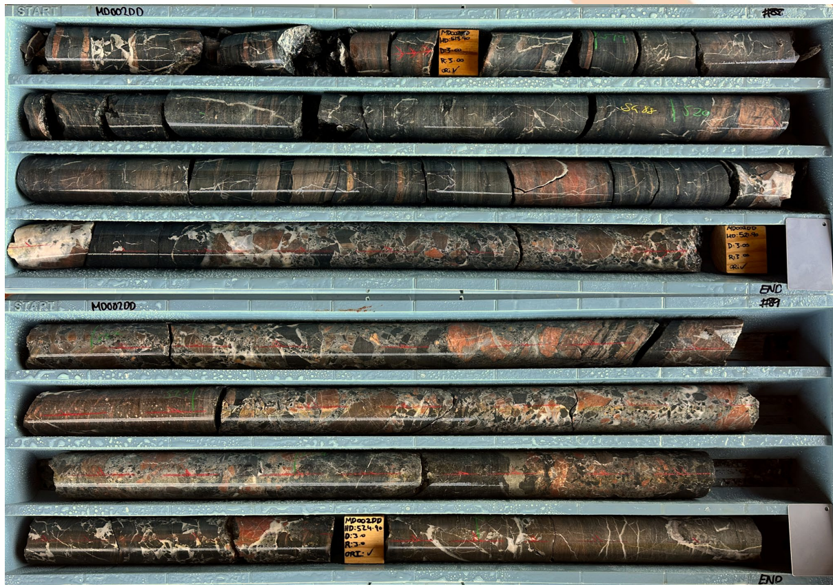
Figure 3: MD002DD HQ core from ~518.5 metres to ~525.2 metres depth showing veining quartz-pyrite throughout with strongly developed hydrothermal breccia textures evident from 521.2 metres to 524.9 metres.
