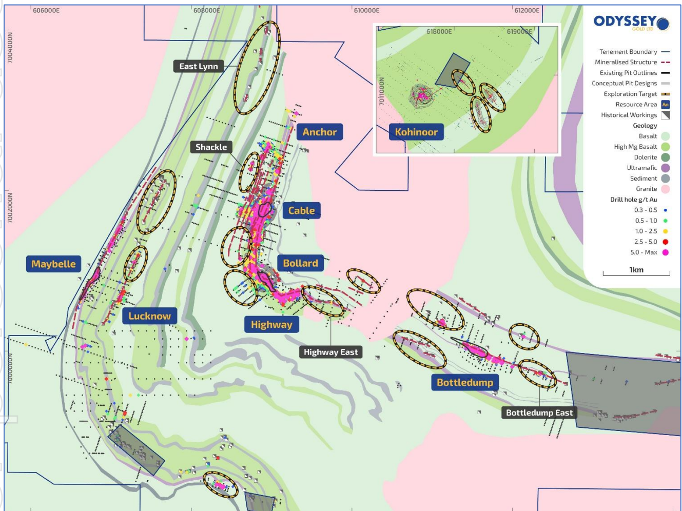
Figure 6 – Tuckanarra Project plan showing priority exploration targets capable of delivering additional MRE growth to support future expansion of the Tuckanarra Project.
