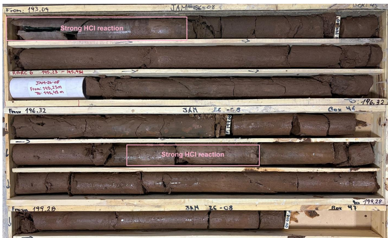
Figure 2. Black sands encountered at 189-200m depth.
