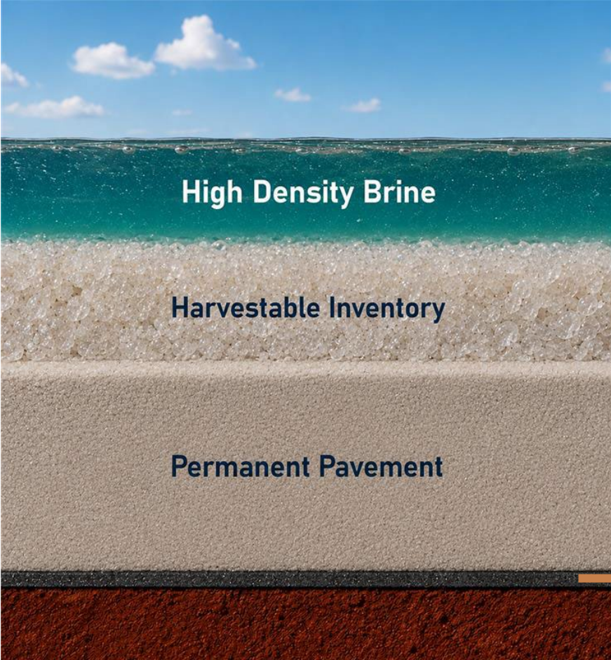
Graphic representation of Mardie crystalliser cross section
