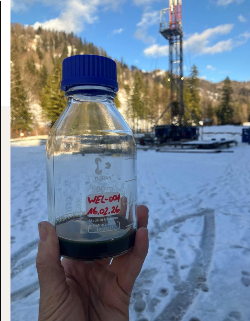
Oil recovered at surface during Reifling Fm testing
