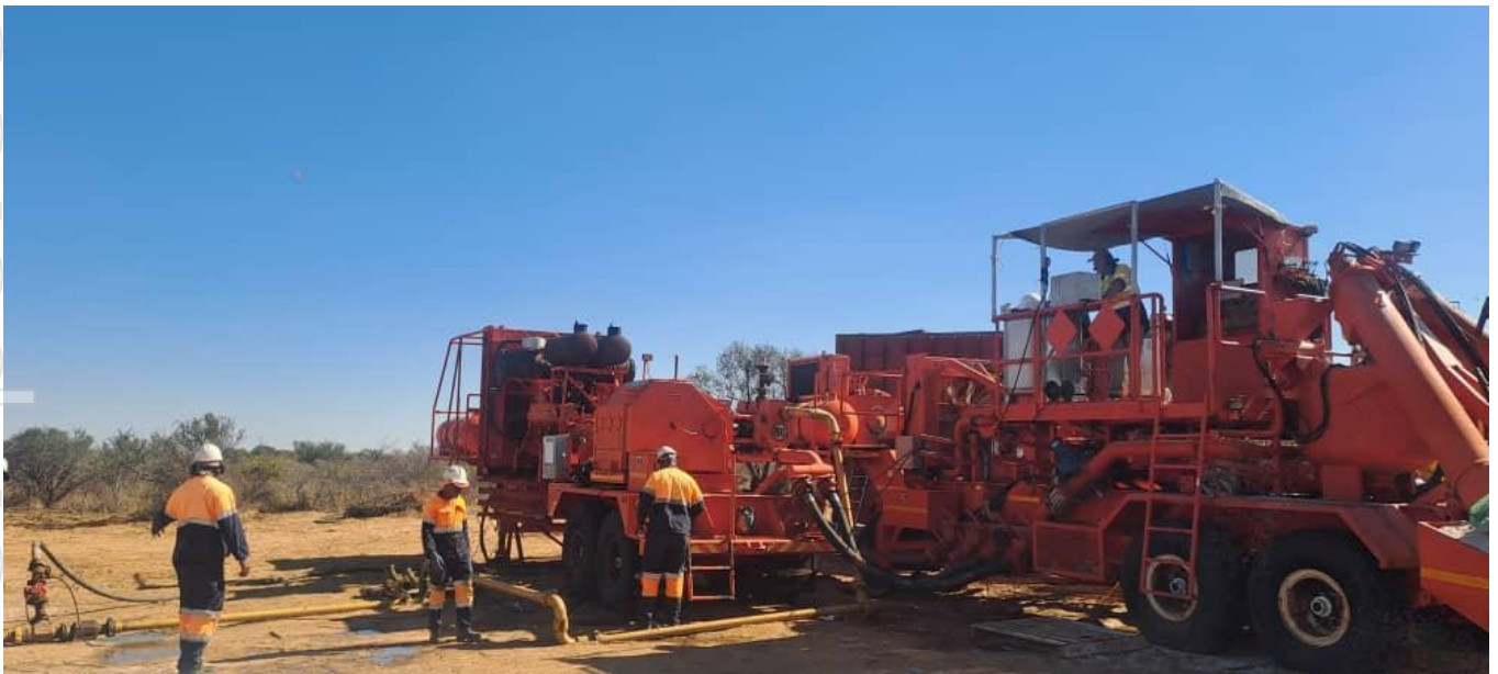
Figure 2. Stimulation units on site at Pitse Pilot well 3.5B (SOURCE: Botala).
