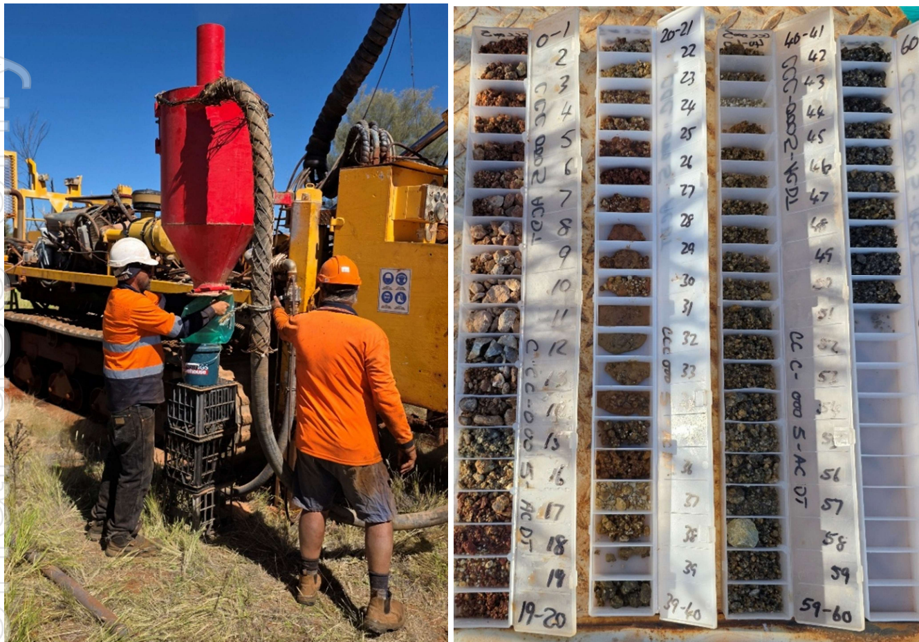
Figure 5A and 5B Air-core chip sample collected through the cyclone and recorded in chip trays for geological logging.
