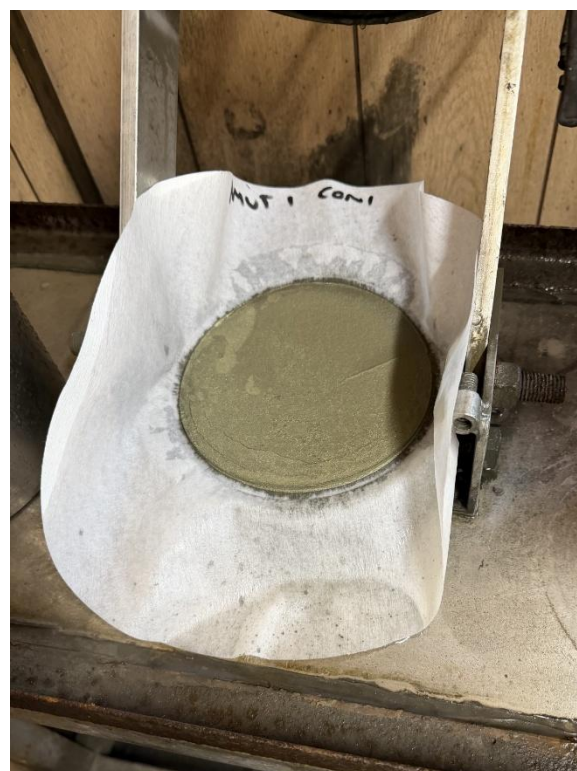
Figure 7: Mutooroo Cu concentrate from preliminary metallurgical test work
