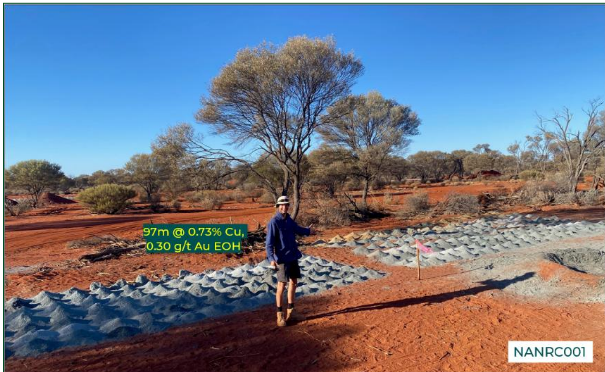
Photo 2. Typical RC drill samples (NANRC001) 2 at Nanadie. Note the limited oxidation profile below shallow sandy soils.
