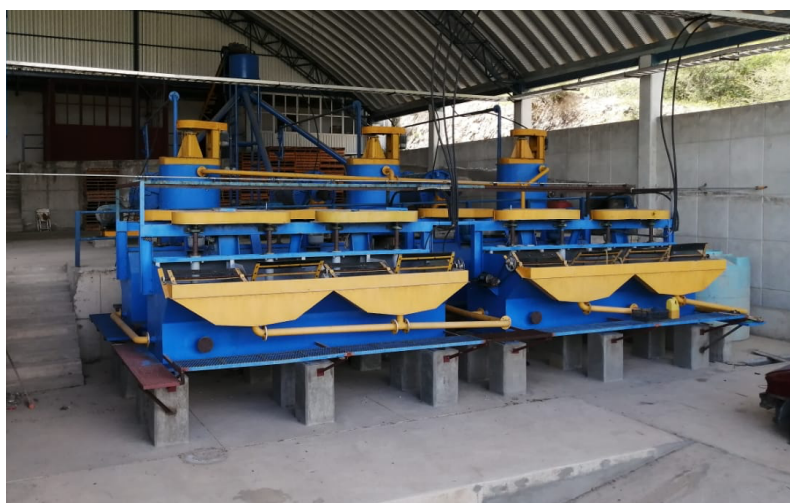
Figure 1. Flotation Cell Banks at Tecmatlán
